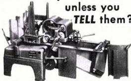
This Elliott Cardvertiser is the only machine in the world that both prints and addresses Post Cards and will address anything at a speed of 100 different addresses per minute.
